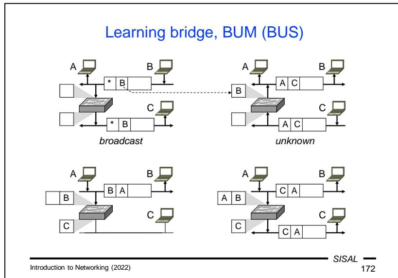
Switches typically operate in the so-called **learning bridge** mode. It means that for each port, they maintain a MAC address table of stations that are connected behind that port and maintain the table themselves by monitoring the traffic.
