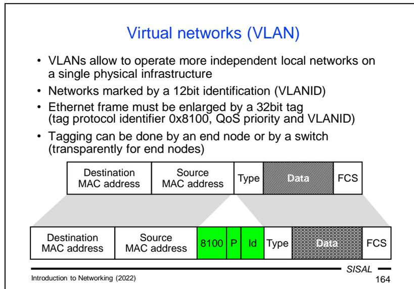
Ethernet version 2 frame format has enabled the deployment of an important network building tool, namely **virtual networks** (VLAN, Virtual LAN). It is used when one physical network needs to be split into multiple logical networks (e.g. when it is shared by multiple entities, or we want to separate segments with a different level of protection).
