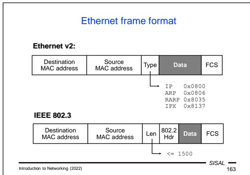
The long and turbulent evolution of Ethernet has also affected the structure of its frame format. While in the original concept the header contains a two-byte type of network protocol behind MAC addresses, in the IEEE version a frame length is in place and only behind it is the special added LLC header (IEEE 802.2).
