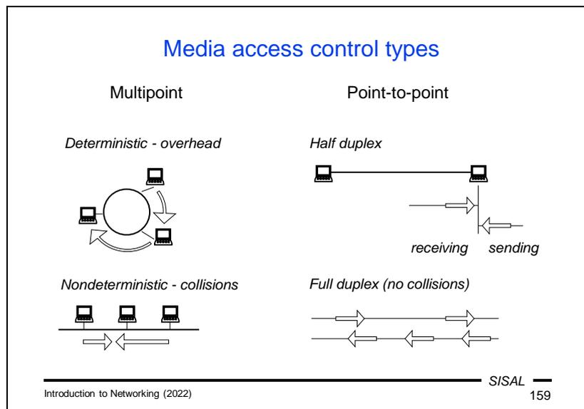
Network topology largely determines the capabilities of a given technology in terms of managing the access of nodes to a medium, so that the technology can cope with parallel transmission requirements.
