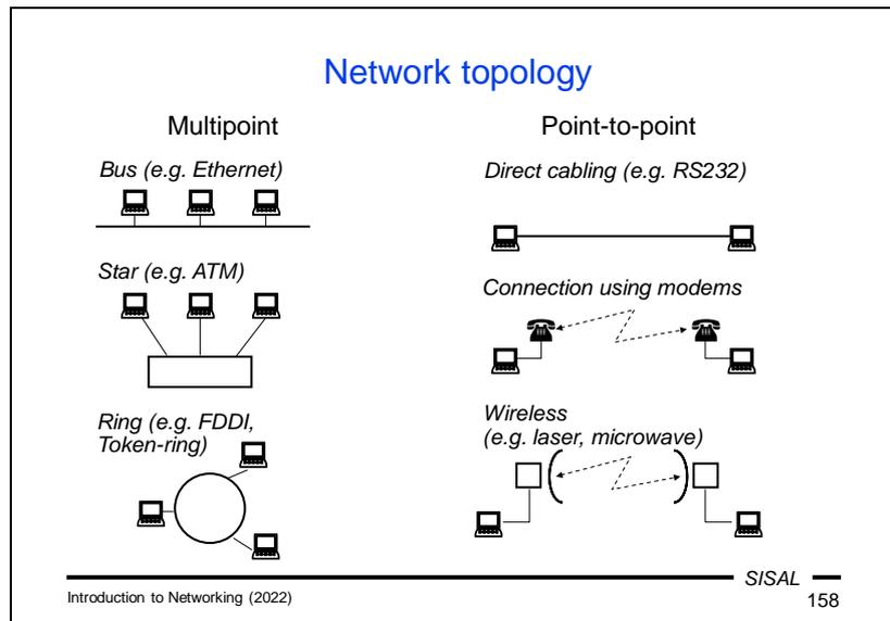
One of the criteria for classification of various technologies of the lower two OSI layers are their topology schemas (arrangement of nodes). A network topology can be studied from either a **physical** perspective, i.e. how the nodes are actually connected (e.g. by cable), or a **logical** one (how the nodes communicate with each other).
