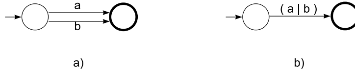
Figure 5.9: An example of collapsing transitions. a) an automaton before collapse b) an automaton after collapse
