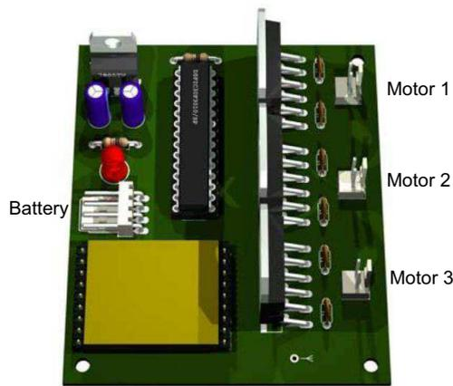
Fig. 2. Electronic board used to control the robot.
